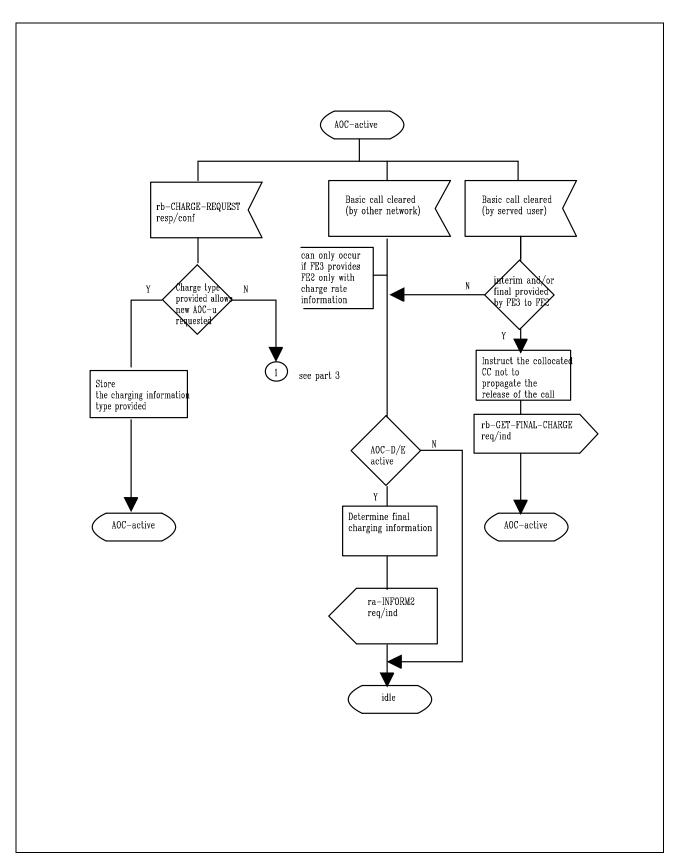
Figure 22 (part 5) - SS-AOC, SDL for functional entity FE2
