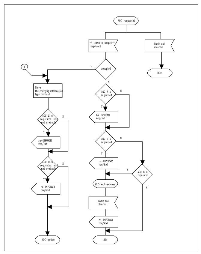
Figure 22 (part 3) - SS-AOC, SDL for functional entity FE2
