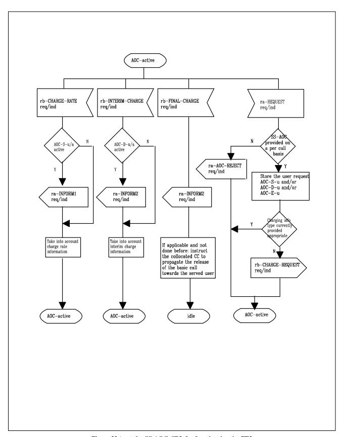
Figure 22 (part 4) - SS-AOC, SDL for functional entity FE2
