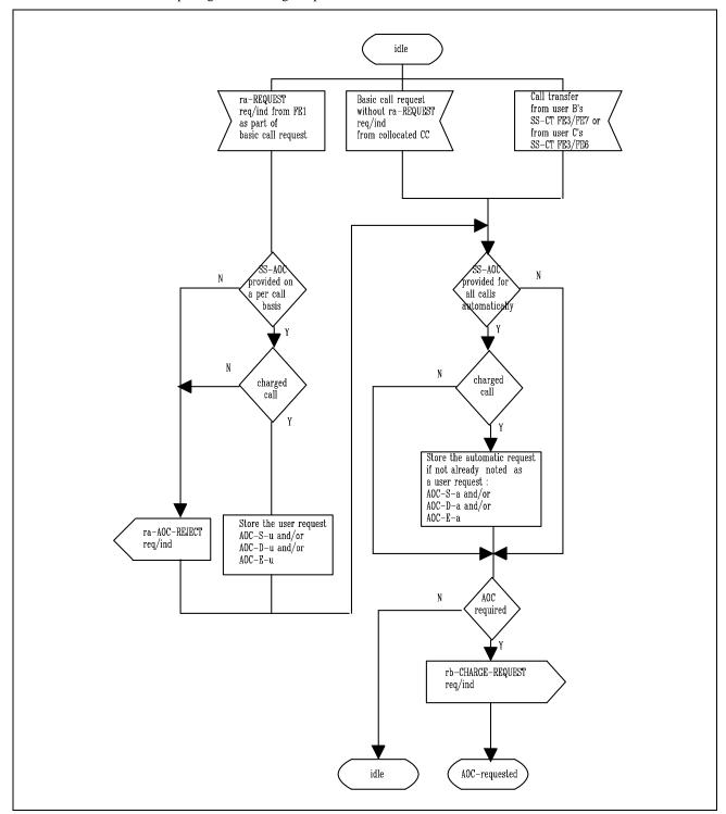
Figure 22 (part 1) - SS-AOC, SDL for functional entity FE2
