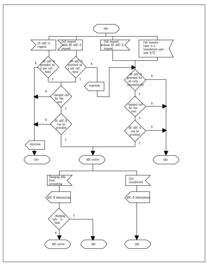
Figure 2 - SS-AOC-D, overall SDL
