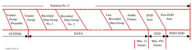
Figure 57 - Layout of a partitioned tape
