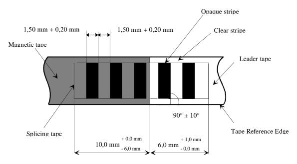
Figure 29 - Splicing tape at PBOT
