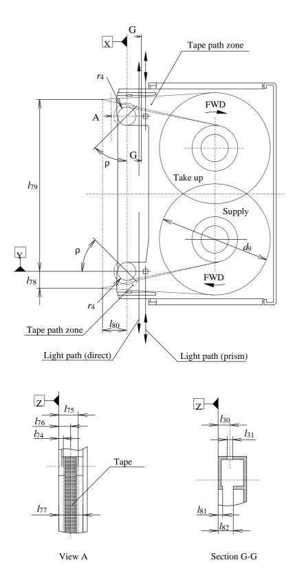
Figure 12 - Inside view of the lower half
