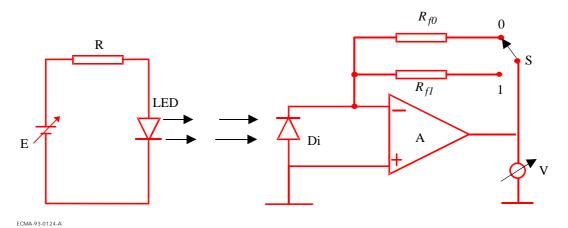
Figure B.2 - Measuring circuitry
