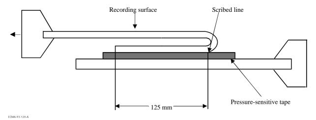
Figure 27 - Measurement of coating adhesion
