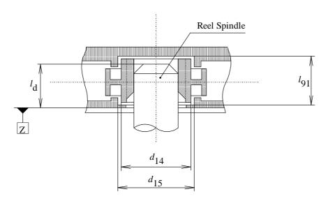
Figure 17 - Interface with the drive spindle
