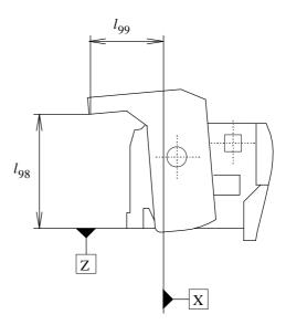
Figure 20 - Minimum position of the lid for which the hubs are completely unlocked
