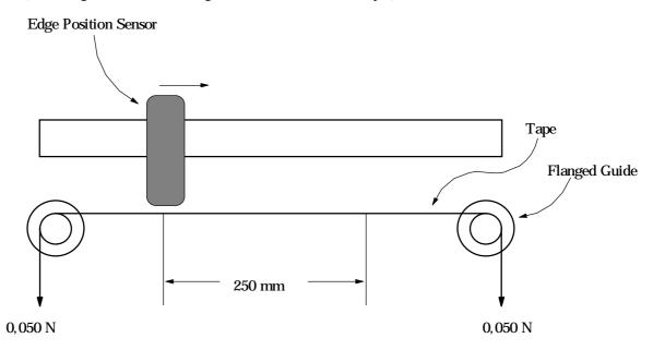
Figure 25 - Measurement of edge weave
