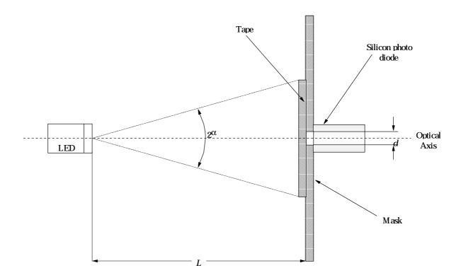
Figure B.1 - Optical arrangement
