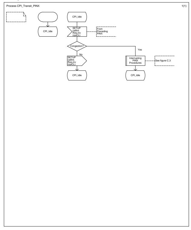
Figure C.2 (sheet 1 of 1) - Transit PINX SDL (SS-CPI)
