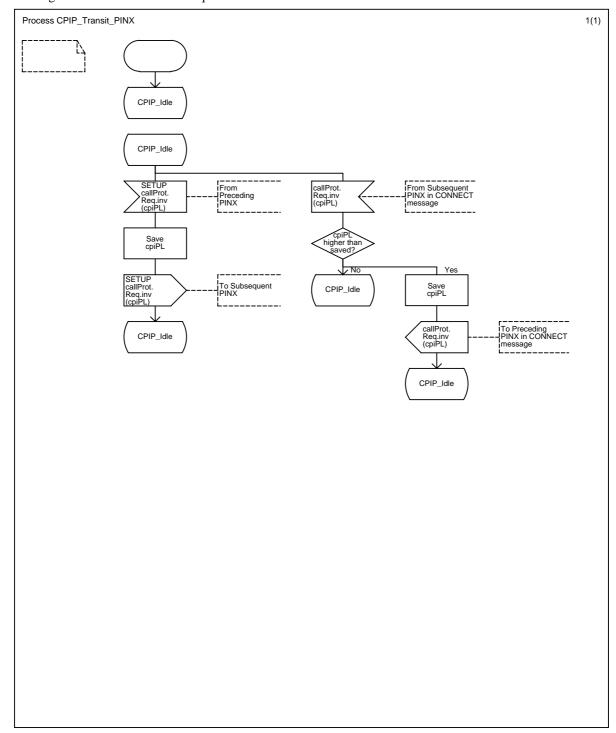
Figure C.5 (sheet 1 of 1) - Transit PINX SDL (SS-CPIP)
