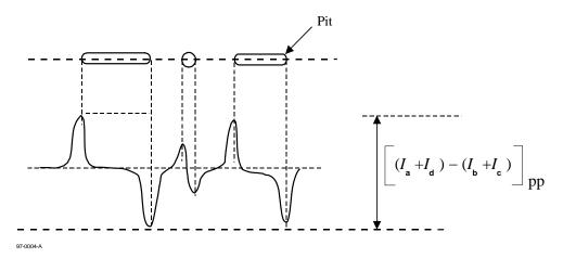
Figure 15 - Tangential push-pull signal
