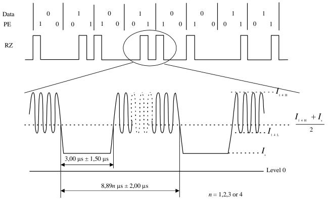
Figure H.4 - Read-out signal from the BCA
