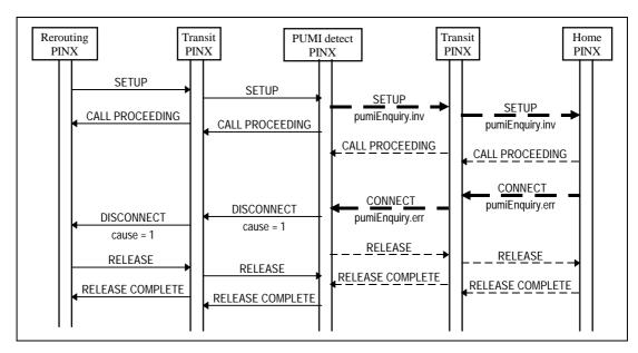
Figure C.3 - Example of ANF-PUMI failure due to PUM user unknown
