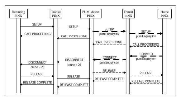
Figure C.4 - Example of ANF-PUMI failure due to PUM user having de-registered
