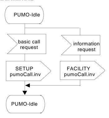
Figure D.5 - Originating PINX behaviour
