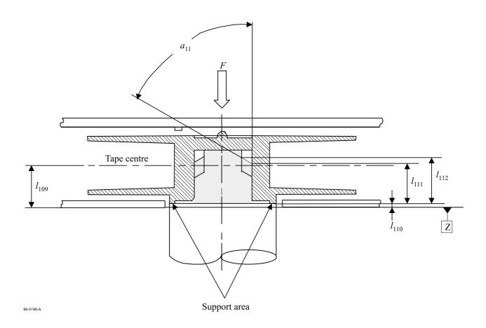
Figure 23 - Interface with the drive spindle
