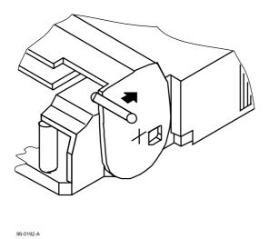
Figure 19 - Direction of the force needed to open the lid
