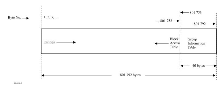
Figure 29 - Structure of a Basic Group
