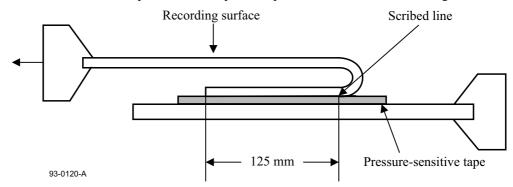
Figure 27 - Measurement of the coating adhesion
