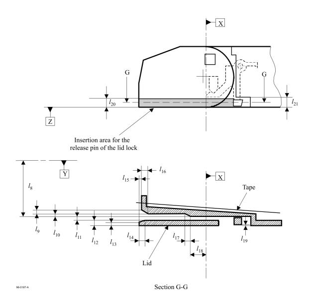
Figure 14 - Lid release insertion channel
