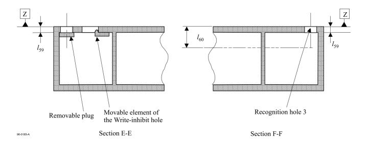
Figure 12 - Cross-sections showing the light path hole, the Recognition and Write-inhibit holes
