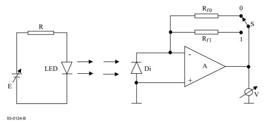
Figure A.2 - Measuring circuitry
