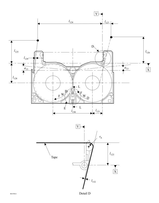
Figure 21 - Internal tape path and light path
