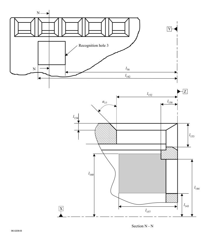
Figure 26 - MIC access holes, enlarged partial view, bottom side
