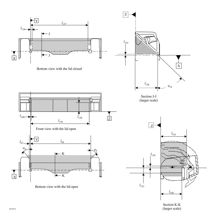
Figure 24 - Tape access cavity clearance
