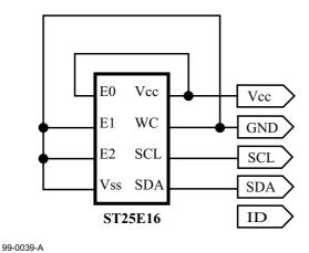
Figure L.1 - Correspondence between Access Holes and chip contacts
