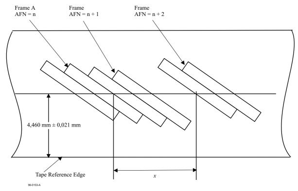
Figure 46 - Tolerance on seamless appending
