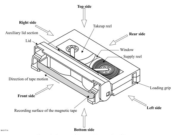
Figure 1 - Tape cartridge assembly, top view, lid open
