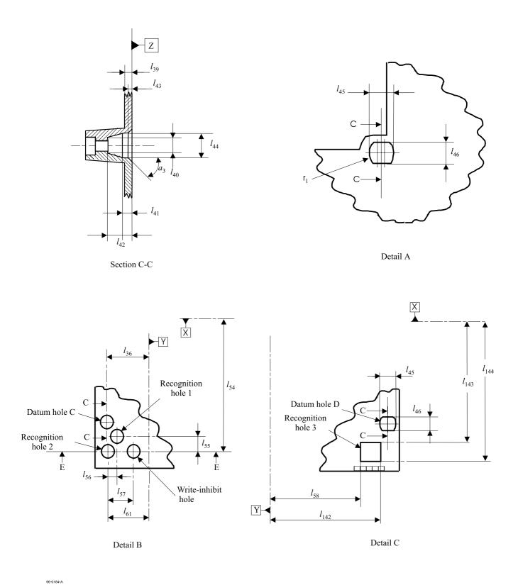
Figure 11 - Details of the Datum, Recognition and Write-inhibit holes
