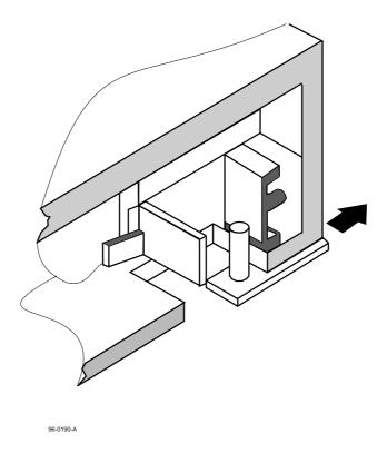
Figure 17 - Direction of the force needed to unlock the reel lock
