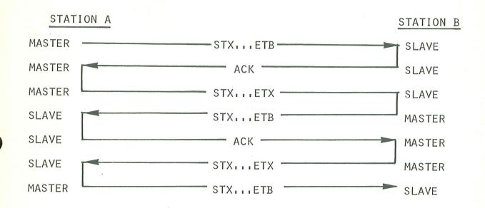
FIG.2 RECOVERY PROCEDURE
