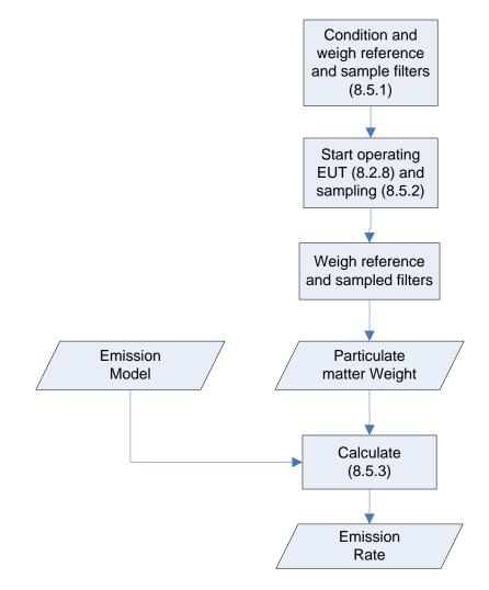
Figure 4 — Determination method for particulate matter
