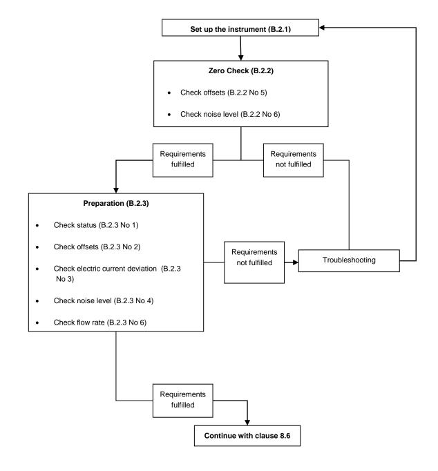
Figure B.1 — Scheme for the operational readiness test for Fast AMS
