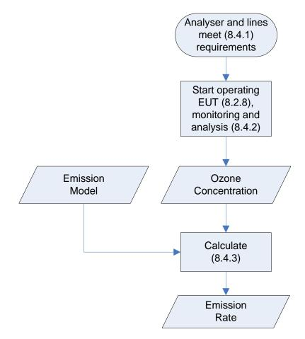
Figure 3 — Determination method for ozone
