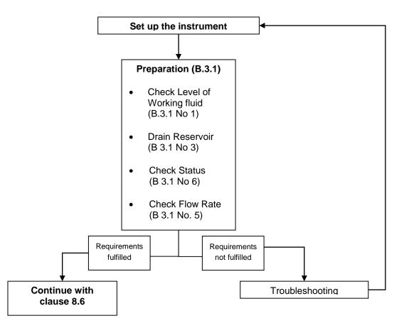
Figure B.2 — Preparation scheme for CPC
