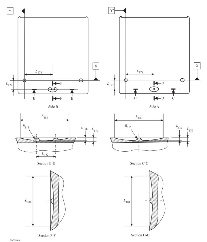
Figure 36 - Identification marks of Side A and B
