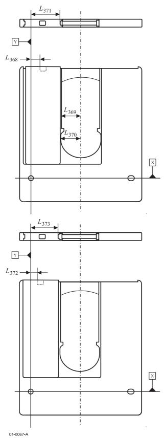
O1-0067-A Figure 45 - Shutter in just open position (top view) and maximum open position (bottom view)
