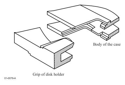
Figure J.2 - Connection between grip of disk holder and body
