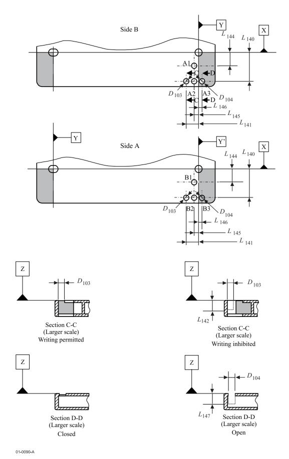
Figure 9 - Write-inhibit hole, sensor holes and sensing areas
