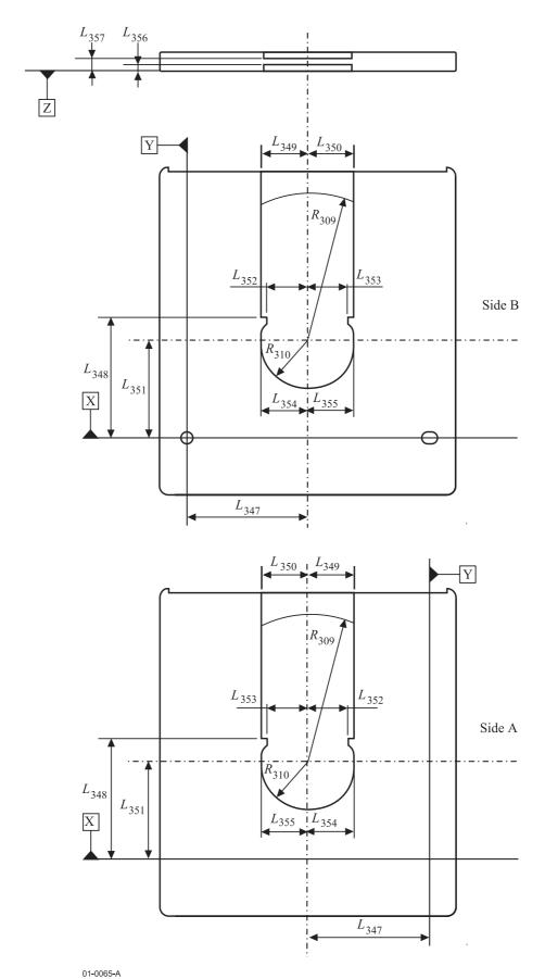
Figure 43 - Spindle and head window
