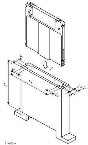
Figure B.1 - Distortion gauge
