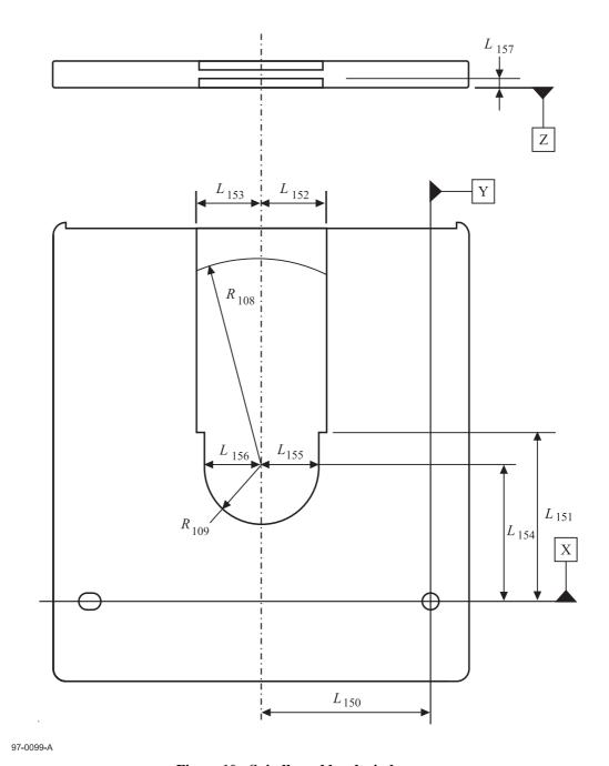
Figure 10 - Spindle and head window
