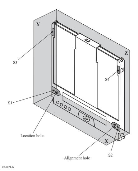
Figure D.1 - Position of the case
