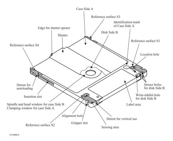
Figure 1 - General view of the Type 1 case, seen from Side A  $\,$
