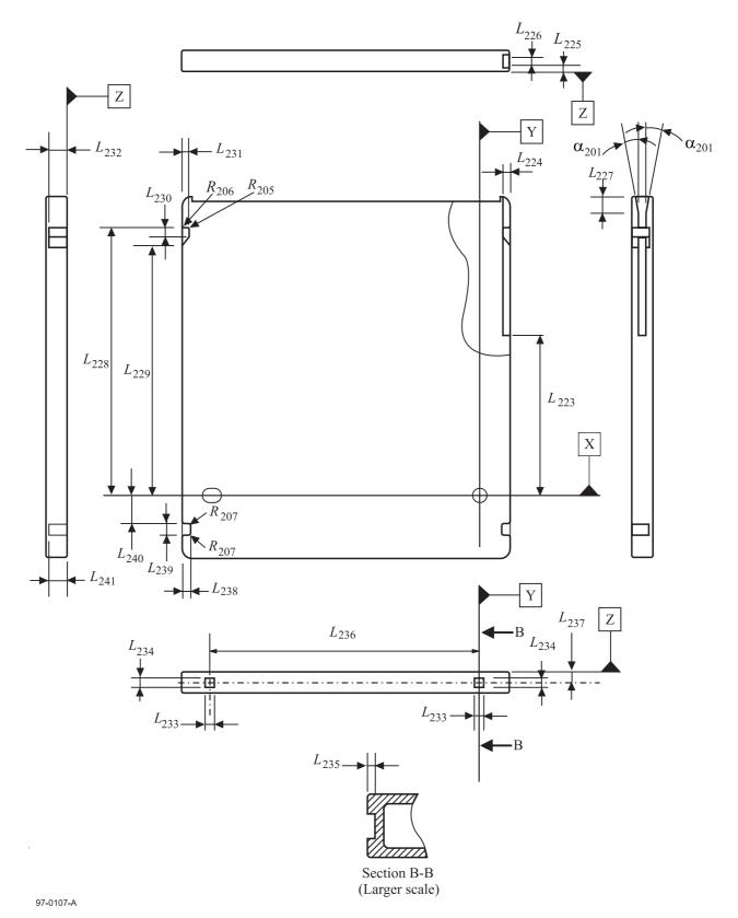
Figure 18 - Insertion slot, detents and gripper slots
