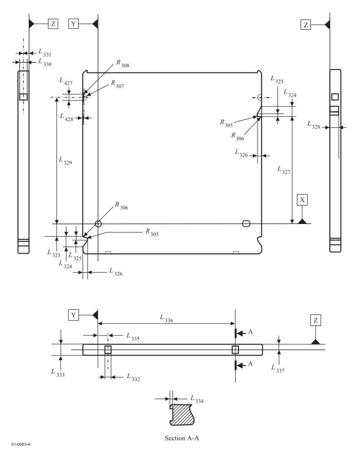
Figure 41 – Mis-insertion protection slot and detents
