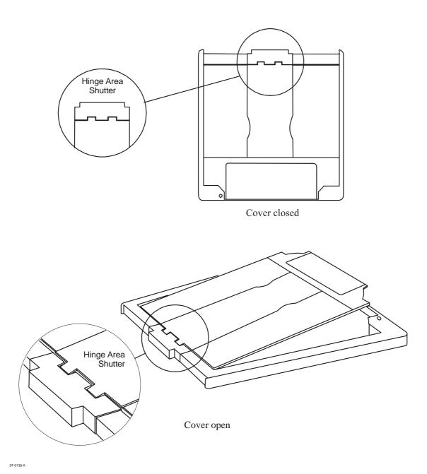
Figure H.2 - Second example of an opening cover
