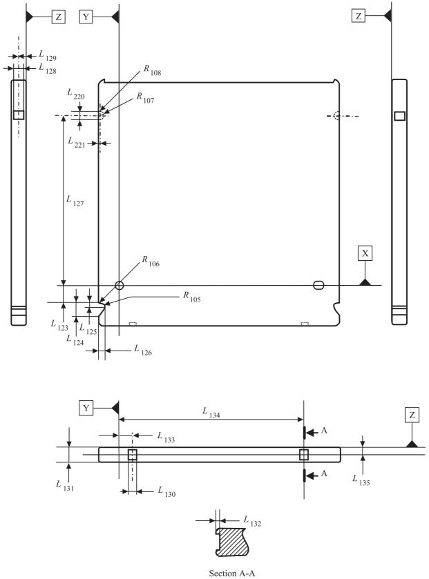
Figure 30 – Mis-insertion protection slots and detents
