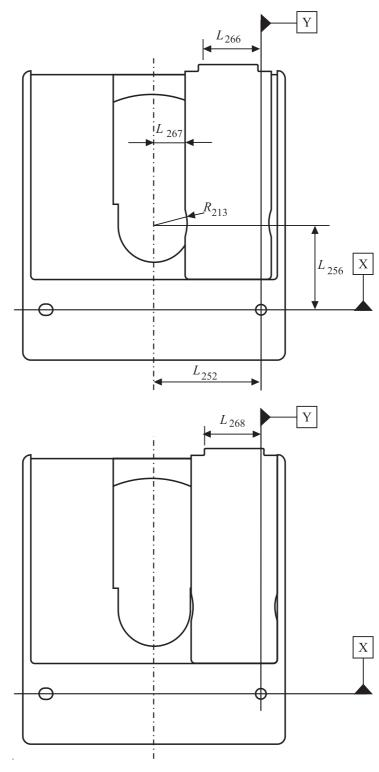
97-0111-A Figure 22 - Shutter in just right-hand open position (top view) and maximum right-hand open position (bottom view)
