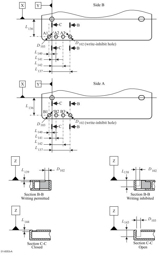
Figure 31 - Write-inhibit hole and sensor holes
