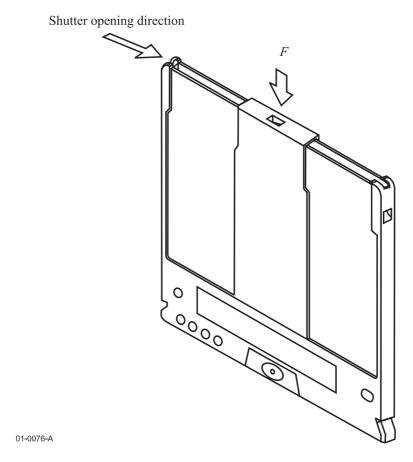
Figure G.1 - Measuring method of shutter opening force
