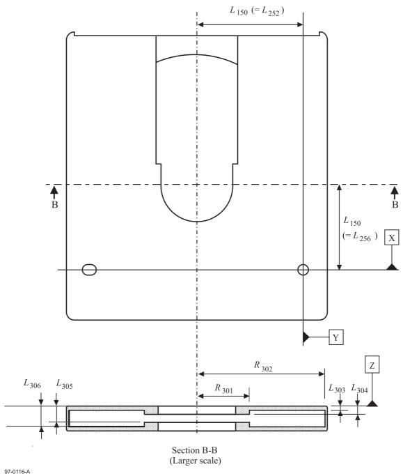
Figure 27 - Inner dimensions of the case
