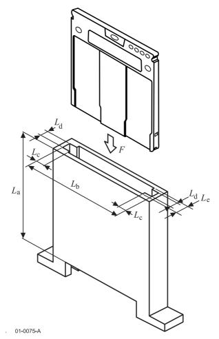
Figure E.1 - Distortion gauge
