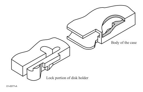
Figure J.1 - Connection between lock portion of disk holder and body
