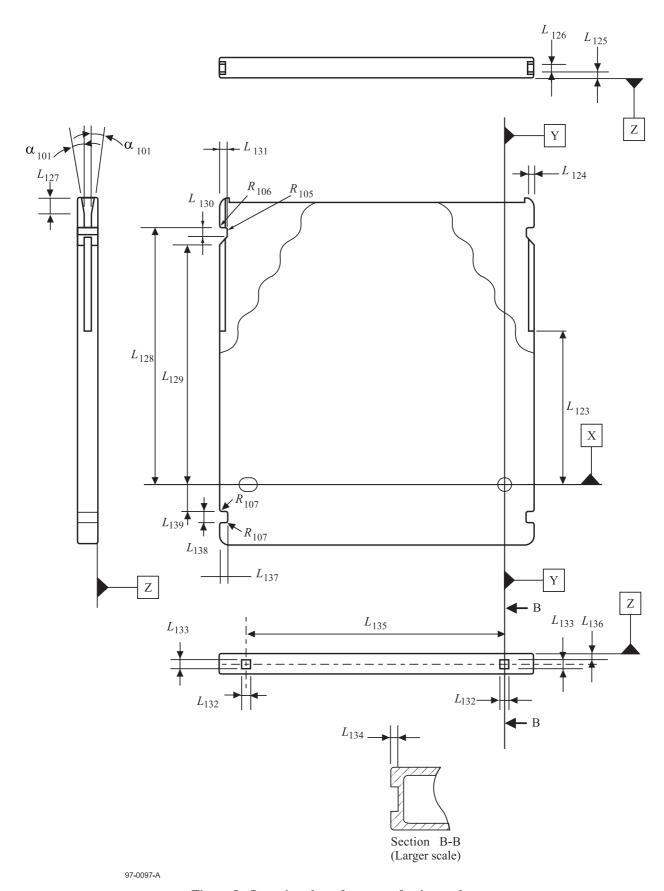
Figure 8 - Insertion slots, detents and gripper slots
