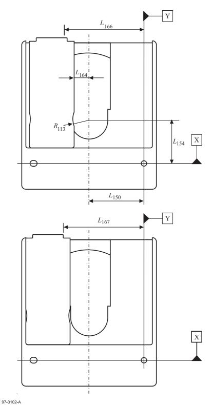
Figure 13 - Shutter in just left-hand open position (top view) and maximum left-hand open position (bottom view)
