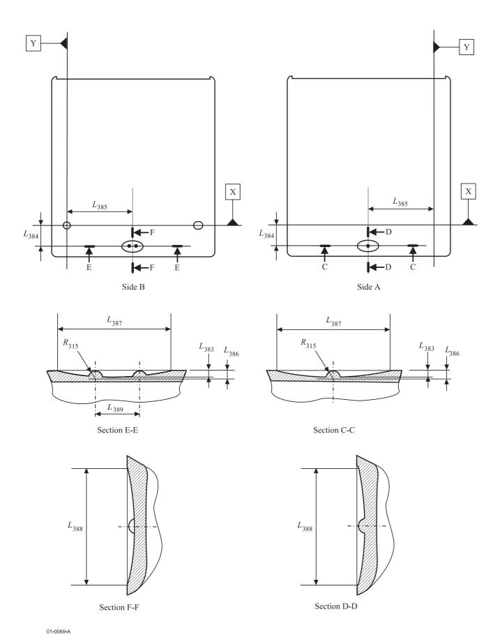
Figure 47 - Identification mark of Side A and B
