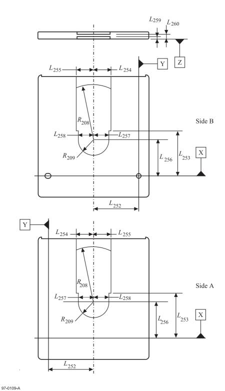
Figure 20 - Spindle and head window
