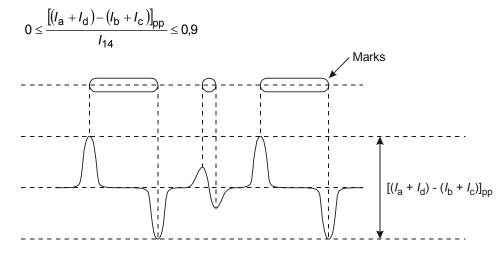
Figure 30 — Tangential push-pull signal
