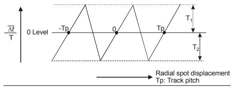
Figure 29 — Differential phase tracking error signal
