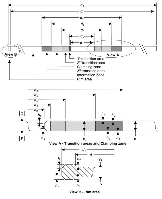
Figure 6 — Physical disk dimensions
