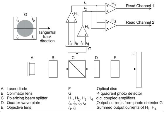
Figure 2 — Optical system of the Reference Drive
