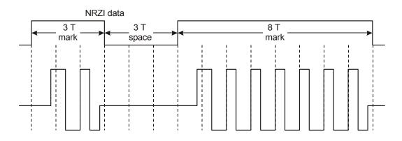
Figure G.2 — Example of a Multiple-pulse
