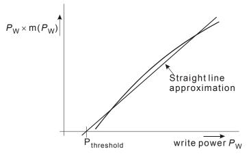
Figure I.2 — Modulation times Power versus Power function
