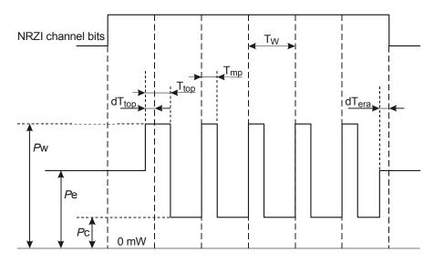
Figure G.1 — Write pulse waveform
