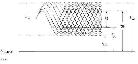
Figure 27 — Signals from spaces and marks in Read channel 1
