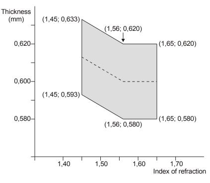
Figure 8 — Thickness of the substrate
