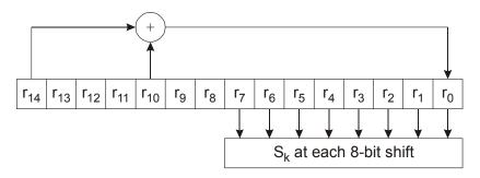
Figure 12 — Feedback shift register
