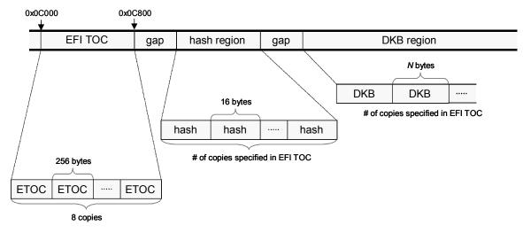
Figure B.1 — Example lay-out of Extended format information in ADIP
