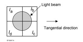
Figure 28 — Quadrant photo detector
