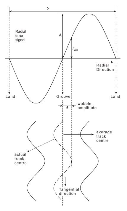
Figure K.1 — Wobble amplitude of the groove
