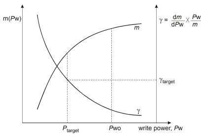
Figure I.1 — Modulation and Gamma functions versus power
