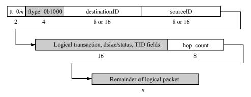
Figure 1-4. Maintenance Packet Transport Bit Stream
