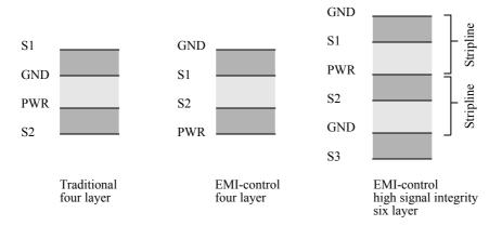
Figure 6-2. Potential PCB Stackups
