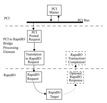
Figure 4-4. PCI Mastered Posted Write Transaction Flow Diagram
