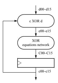
Figure 2-8. CRC Generation Pipeline
