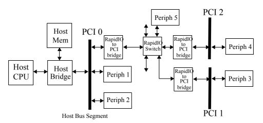
Figure 4-1. Example System with PCI and RapidIO
