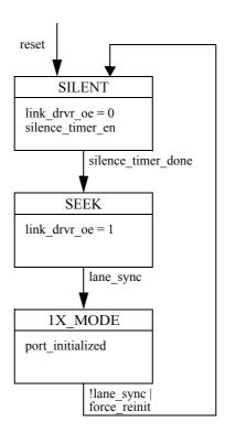
Figure 4-11. 1x\_Initialization State Machine
