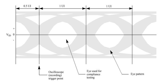
Figure 8-7. Example Receiver Input Eye Pattern
