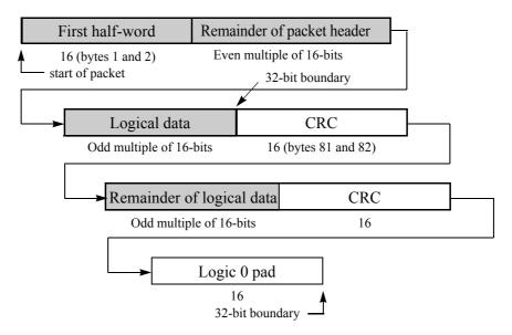
Figure 2-7. Padded Packet of Length Greater than 80 Bytes
