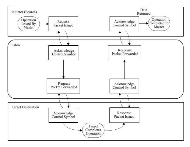
Figure 1-1. Example Transaction with Acknowledge
