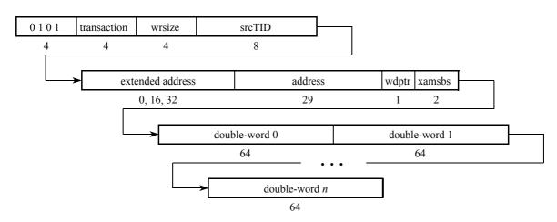
Figure 3-2. Type 5 Packet Bit Stream Format
