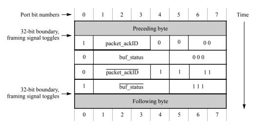
Figure 3-8. Control Symbol Transmission Example 1
