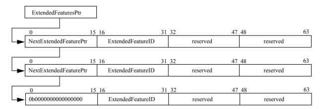
Figure 4-1. Example Extended Features Data Structure
