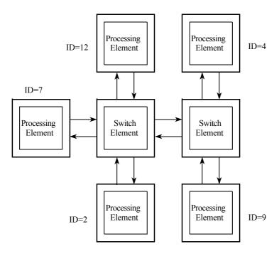
Figure 1-1. A Small Switch-Based System
