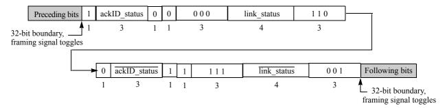
Figure 3-6. Type 6 Link-Response Control Symbol Format
