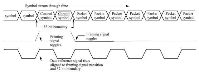
Figure 2-2. Framing Signal Maximum Toggle Rate for 16-bit Port
