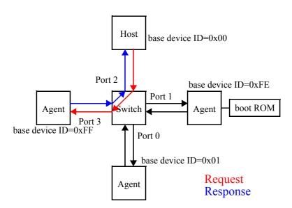
Figure 2-7. Finding the device on switch port 3
