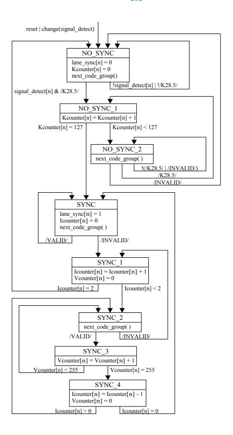
Figure 4-9. Lane\_Synchronization State
