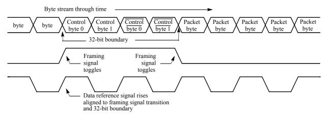
Figure 2-1. Framing Signal Maximum Toggle Rate for 8-bit Port
