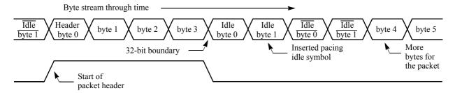
Figure 2-7. Pacing Idle Insertion in Packet (8-bit Port)
