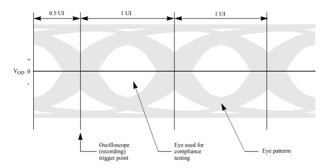
Figure 8-5. Example Driver Output Eye Pattern
