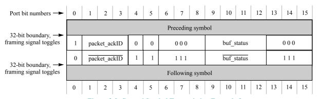
Figure 3-9. Control Symbol Transmission Example 2
