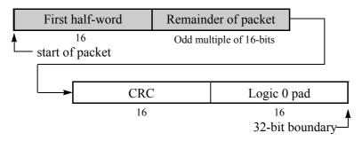
Figure 2-5. Padded Packet of Length 80 Bytes or Less
