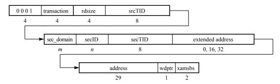
Figure 4-1. Type 1 Packet Bit Stream Format
