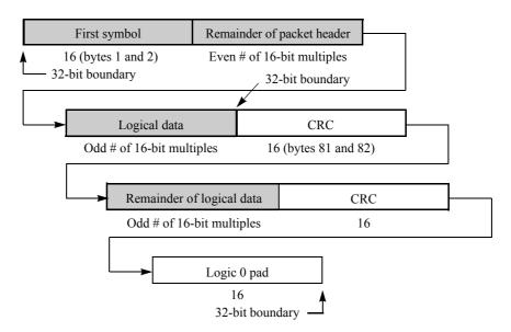
Figure 1-12. Padded Aligned Packet Bit Stream Example 2
