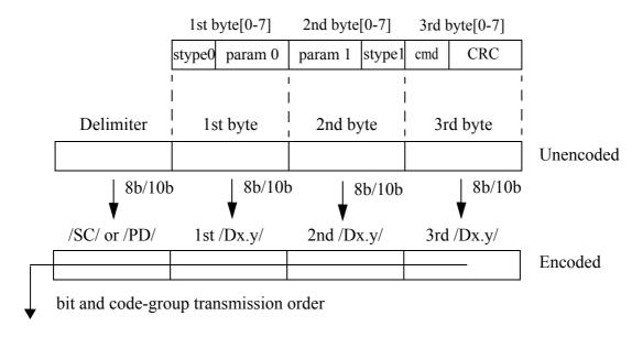
Figure shows the encoding and transmission order for a packet transmitted over a 1x LP-Serial link.
