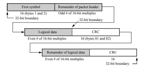
Figure 1-10. Naturally Aligned Packet Bit Stream Example 2
