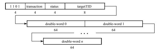
Figure 3-6. Type 13 Packet Bit Stream Format
