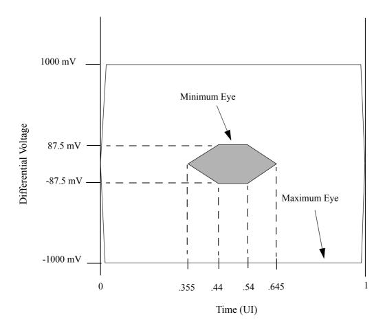
Figure 8-3. 1.25 Gbps Baud Rate Receiver Eye Diagram
