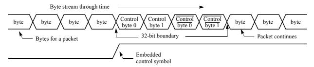
Figure 2-8. Embedded Control Symbols for 8-bit Port
