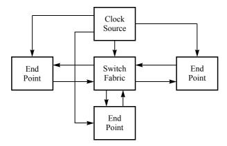
Figure 5-1. Clock Distribution in a Small System
