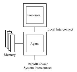
Figure 1-2. Processor-Memory Processing Element Example
