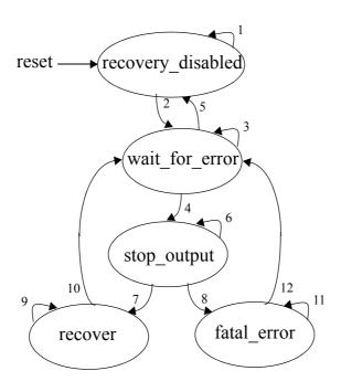
Figure A-4. Output Port Error Recovery State Machine
