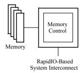
Figure 1-4. Memory-Only Processing Element Example
