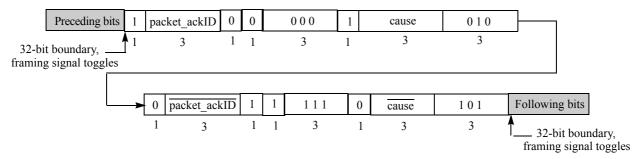
Figure 3-3. Type 2 Packet-Not-Accepted Control Symbol Format
