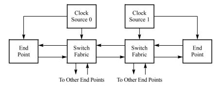
Figure 5-2. Clock Distribution in a Larger System
