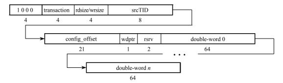
Figure 3-4. Type 8 Request Packet Bit Stream Format
