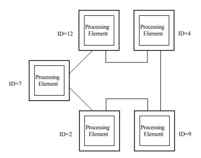
Figure 1-2. A Small Ring-Based System
