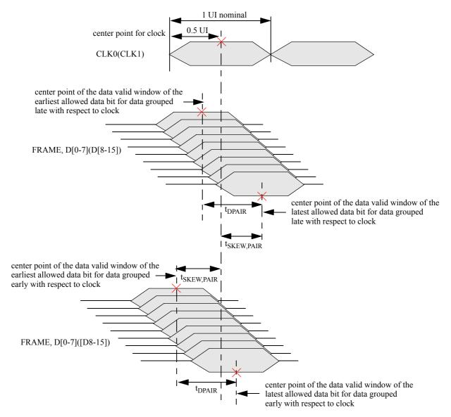
Figure 8-10. Static Skew Diagram
