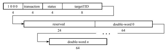
Figure 3-5. Type 8 Response Packet Bit Stream Format
