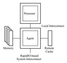
**Figure 2-2 Processor-Memory Processing Element Example**
