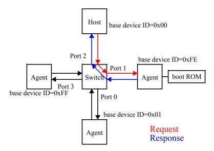
Figure 2-6. Finding the device on switch port 1
