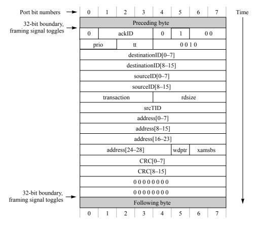
Figure 2-12. Request Packet Transmission Example 3
