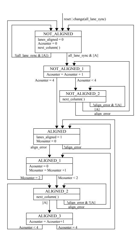
Figure 4-10. Lane Alignment State Machine
