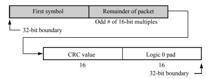
Figure 1-11. added Aligned Packet Bit Stream Example 1
