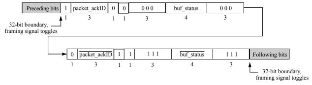
Figure 3-1. Type 0 Packet-Accepted Control Symbol Format
