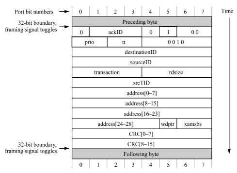
**Figure 2-10. Request Packet Transmission Example 1**
