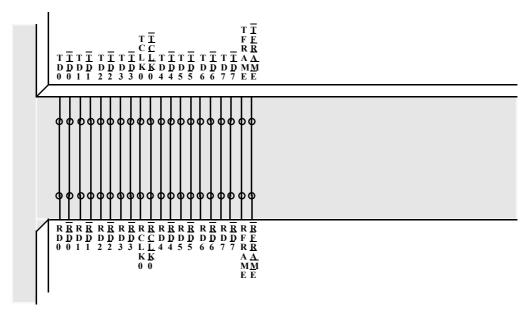
Figure 6-5. Opposed orientation, same side of board
