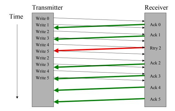
Figure 1-5. Receiver-Controlled Flow Control
