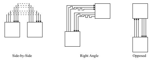
Figure 6-1. Routing for Equalized Skew for Several Placements
