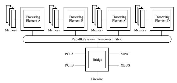
Figure 1-1. A Possible RapidIO-Based Computing System
