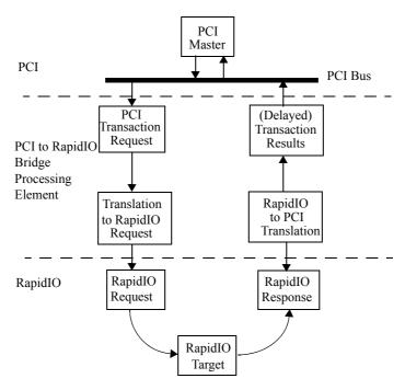
Figure 4-5. PCI Mastered non-posted (delayed) Transaction Flow Diagram
