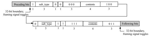
Figure 3-4. Type 4 Packet Control Symbol Format
