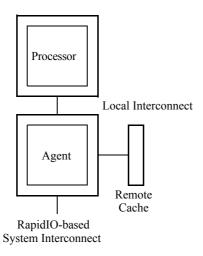
Figure 2-5. Processor-Only Processing Element Example
