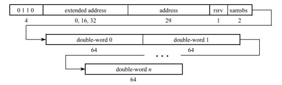
Figure 3-3. Type 6 Packet Bit Stream Format
