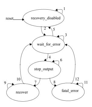
Figure A-6. Output port error recovery state machine
