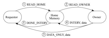
Figure 3-2. Read Operation to Remote Modified Coherence Granule
