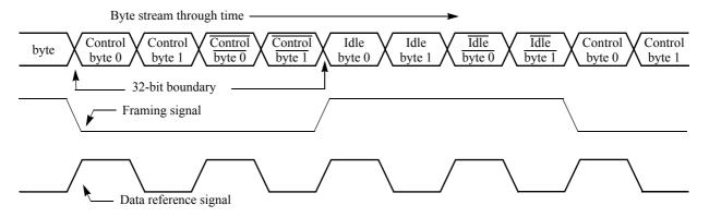
Figure 2-3. Control Symbol Delineation Example for 8-bit Port
