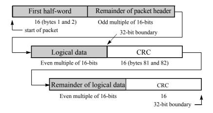
Figure 2-6. Unpadded Packet of Length Greater than 80 Bytes
