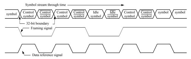
Figure 2-4. Control Symbol Delineation Example for 16-bit Port
