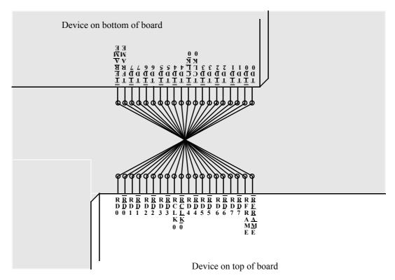
Figure 6-6. Opposed orientation, opposite sides of board
