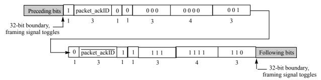
Figure 3-2. Type 1 Packet-Retry Control Symbol Format
