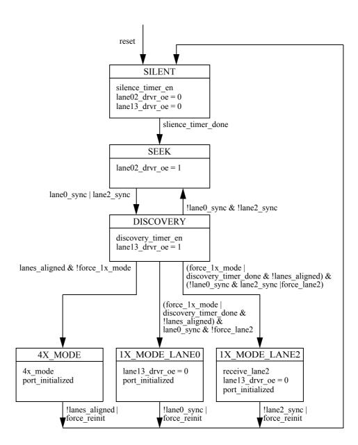
Figure 4-12. 1x/4x Initialization State Machine
