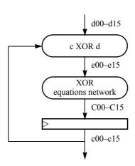
Figure 1-13. CRC Generation Pipeline
