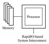
Figure 1-3. Integrated Processor-Memory Processing Element Example
