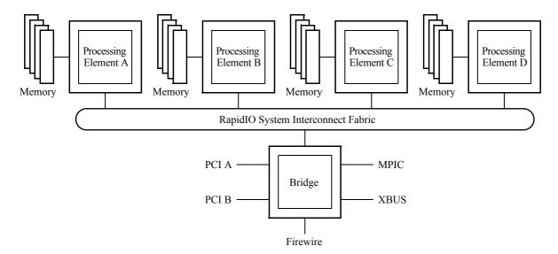
Figure 2-1. A Possible RapidIO-Based Computing System
