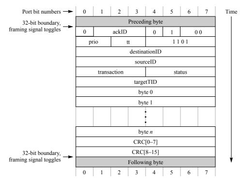
Figure 2-14. Response Packet Transmission Example 1
