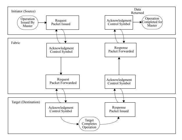
Figure 5-1. Example Transaction with Acknowledgment
