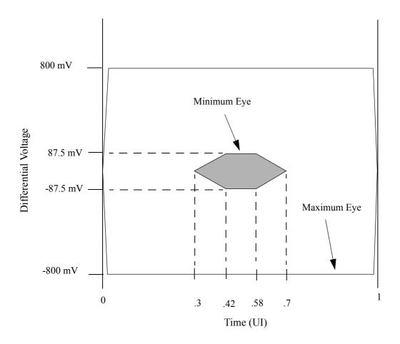
Figure 8-5. 3.125 Gbps Baud Rate Receiver Eye Diagram
