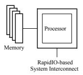
Figure 2-3. Integrated Processor-Memory Processing Element Example
