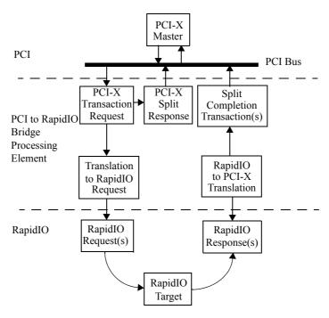
Figure 6-7. PCI-X Mastered Split Response Transaction
