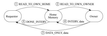
Figure 3-9. Read-for-Ownership Operation to Remote Modified Coherence Granule
