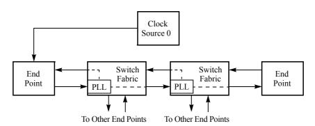
Figure 5-3. Clock Distribution Through the Interconnect
