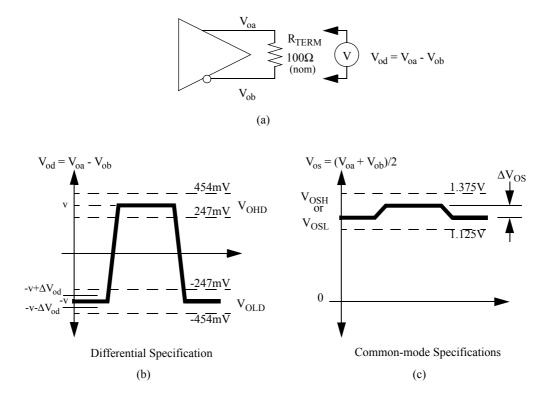
Figure 8-1. DC driver signal levels
