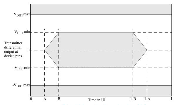
Figure 8-2. Transmitter Output Compliance Mask
