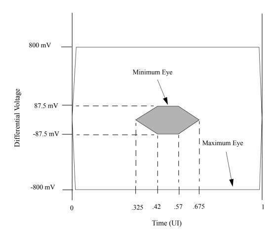
Figure 8.4. 2.5 Gbps Baud Rate Receiver Eye Diagram
