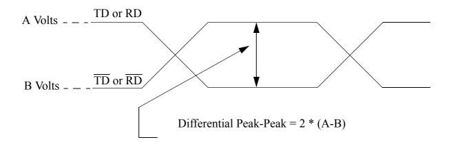
Figure 8-1. Differential Peak-Peak Voltage of Transmitter or Receiver
