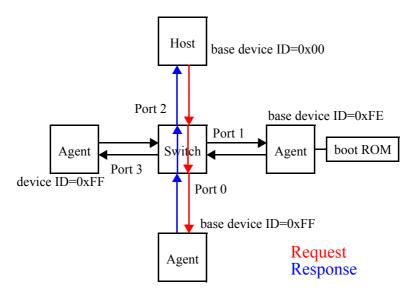
Figure 2-5. Finding the device on switch port 0
