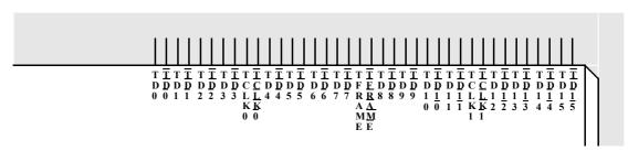
Figure 6-7. Recommended device pin escape, output port reversed, top view of device
