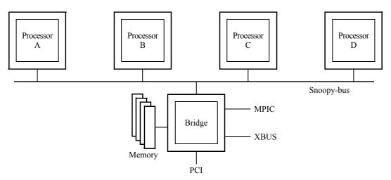
Figure 1-1. A Snoopy Bus-Based System
