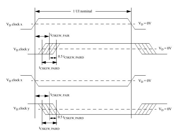
Figure 8-9. Clock to Clock Skew
