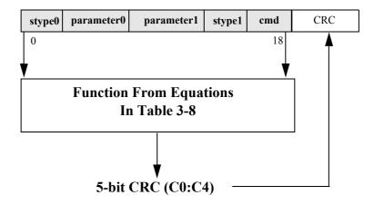
Figure 3-13. 5-bit CRC Implementation4Chapter 4 - PCS and PMA Layers
