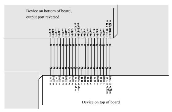
Figure 6-8. Opposed orientation, output port reversed, opposite sides of board
