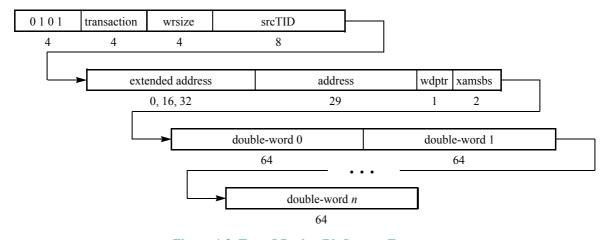
Figure 4-3. Type 5 Packet Bit Stream Format
