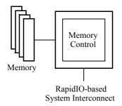
Figure 1-4. Memory-Only Processing Element Example
