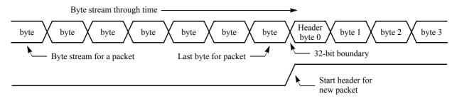
Figure 2-5. Header Marked End of Packet (8-bit Port)
