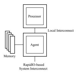
Figure 1-2. Processor-Memory Processing Element Example
