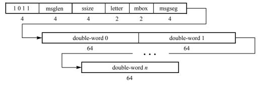
Figure 3-2. Type 11 Packet Bit Stream Format
