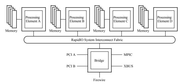
Figure 1-1. A Possible RapidIO-Based Computing System
