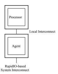
Figure 1-5. Processor-Only Processing Element Example
