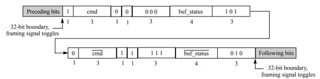
Figure 3-5. Type 5 Link-Request Control Symbol Format
