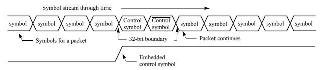
Figure 2-9. Embedded Control Symbols for 16-bit Port
