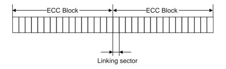
Figure 34- Structure of ECC Block without Linking Loss Area (Lossless-Link)
