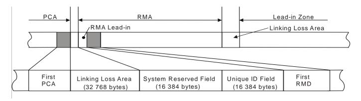
Figure 59 - Layout of the Recording Management Area
