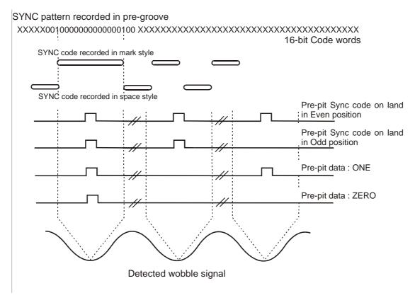
Figure 42 - Relationship of signals recorded in groove and land
