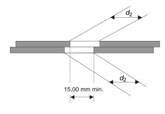
Figure 8 - Hole of the assembled disk
