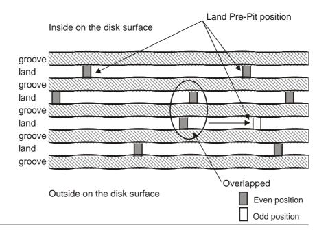
Figure 43 - Layout of land Pre-pit positioning
