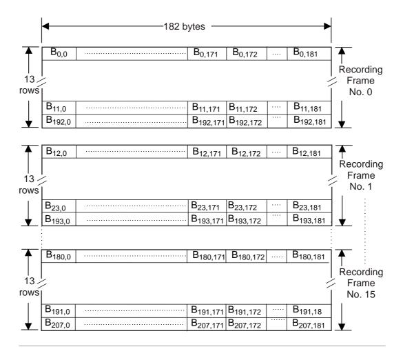
Figure 28 - Recording Frames obtained from an ECC Block
