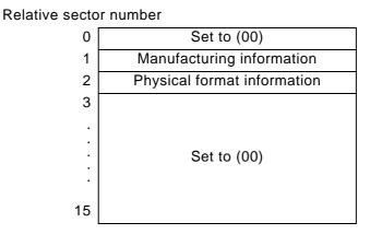
*Figure 37 – Structure of a R-Physical format information block*
