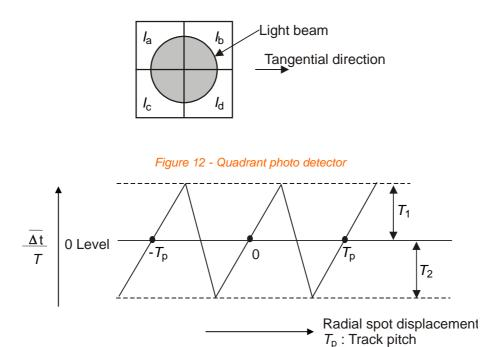
Figure 13 - Differential phase tracking error signal
