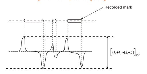
Figure 14 - Tangential push-pull signal
