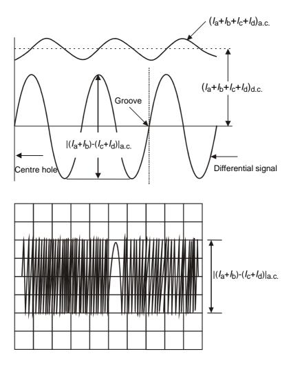
Figure 19 - Radial push-pull tracking error signal
