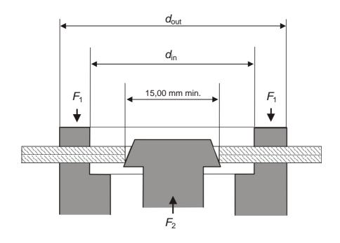
Figure A.2 - Clamping and chucking conditions
