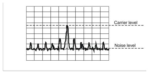
Figure 15 - Measurement of the wobble CNR
