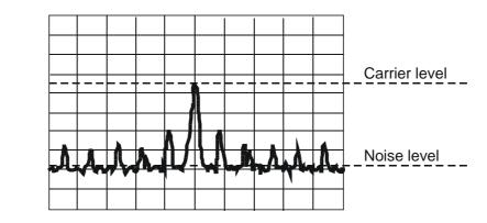
Figure 21 - Measurement of the wobble CNR
