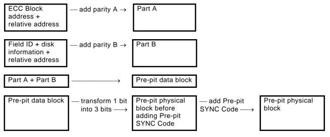
Figure 46 - Processing order to construct a Pre-pit block
