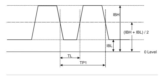
Figure L.3 - Read-out signal from NBCA
