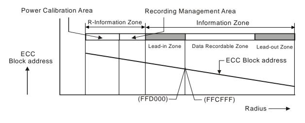
Figure 40 - Pre-pit sector layout and ECC Block numbering
