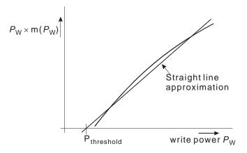
Figure I.2 - Modulation times Power versus Power function
