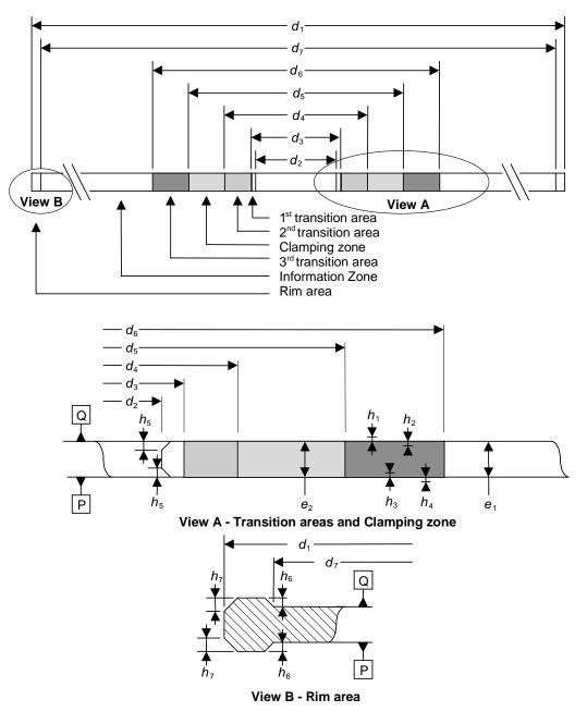
Figure 6 - Physical disk dimensions
