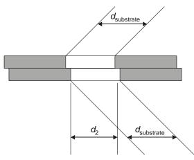
Figure 7 - Hole diameters for an assembled disk
