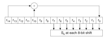
Figure 13 - Feedback shift register
