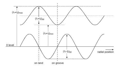
Figure 37 - Signals from grooves in the Read Channels when crossing the tracks
