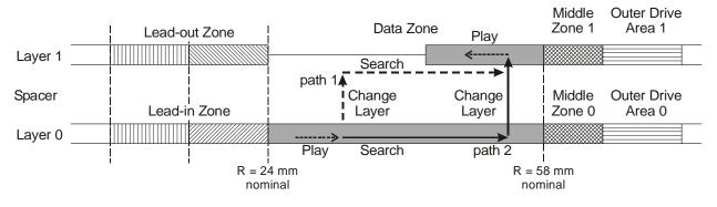
Figure K.1 - Recommended access for a partially recorded Layer 1
