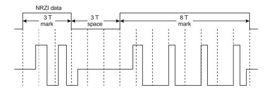
Figure G.4 - Example of a Multiple-pulse
