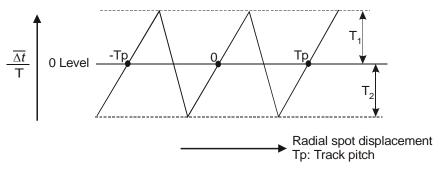
Figure 41 - Differential phase tracking error signal
