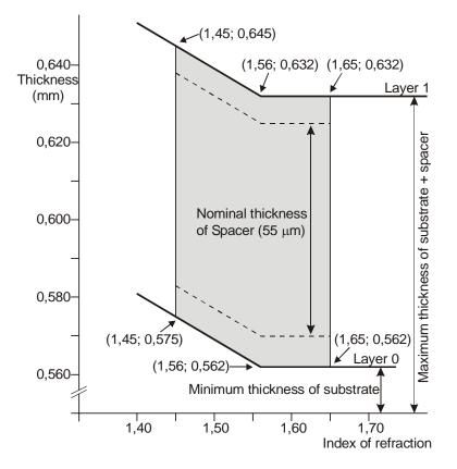
Figure 9 - Thickness of the substrate
