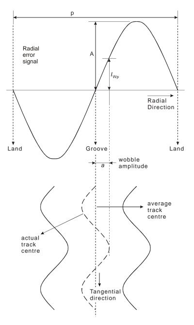
Figure L.1 - Wobble amplitude of the groove
