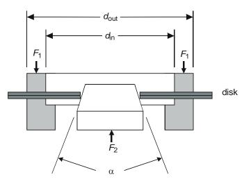
Figure 3 - Clamping and chucking conditions
