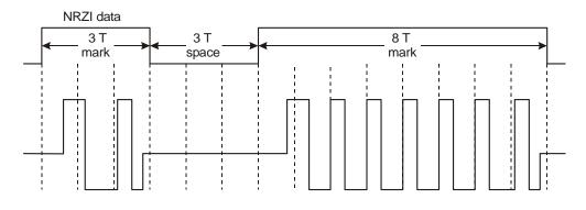
Figure G.2 - Example of a Multiple-pulse
