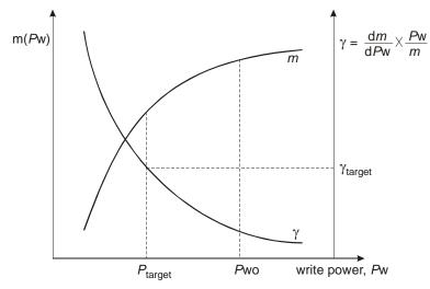
Figure I.1 – Modulation and Gamma functions versus power
