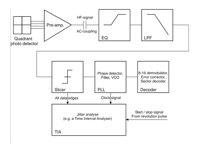
Figure F.1 — General diagram for jitter measurement
