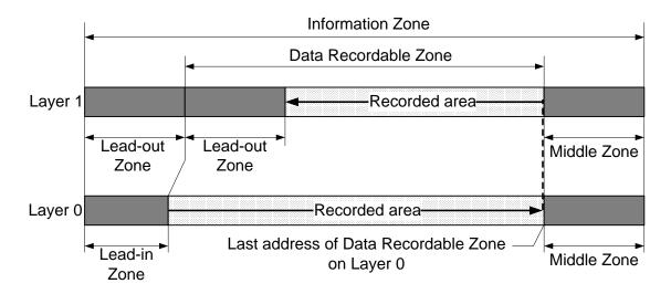
Figure N.1 — Examples of Information Zone with Format1 RMD
