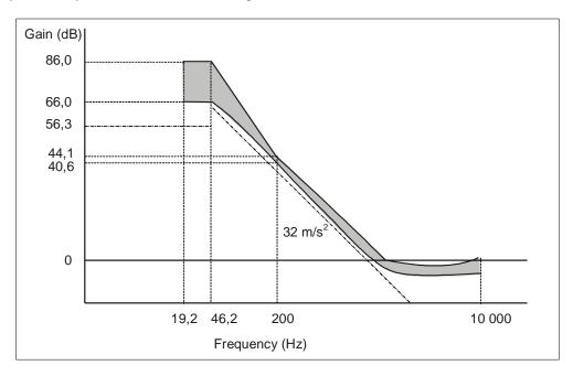
Figure 5 — Reference servo for axial tracking of unrecorded disk
