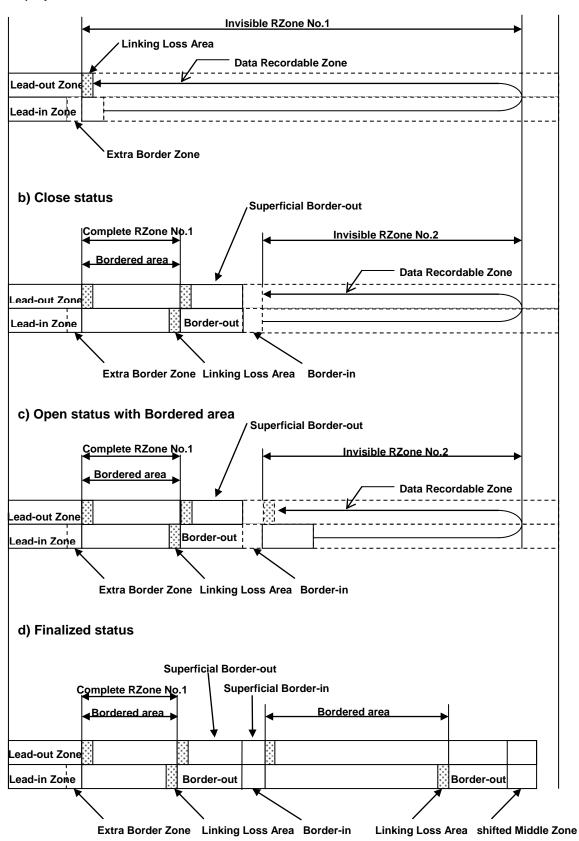
Figure L.2 — Examples of Border Recording in Information Zone
