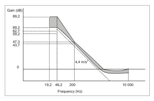
Figure 7 — Reference servo for radial tracking of recorded disk
