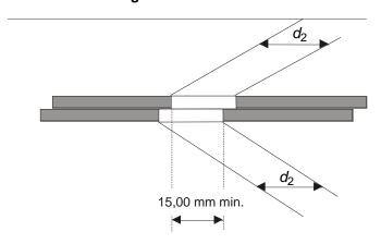
Figure 10 — Hole of the assembled disk
