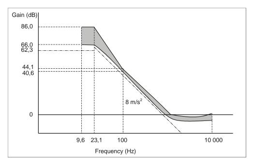
Figure 4 — Reference servo for axial tracking of recorded disk
