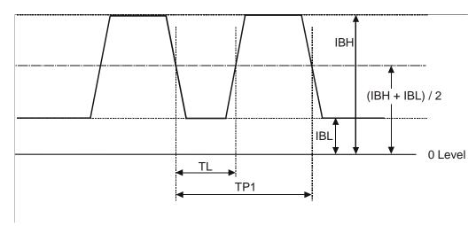
Figure K.3 — Read-out signal from NBCA
