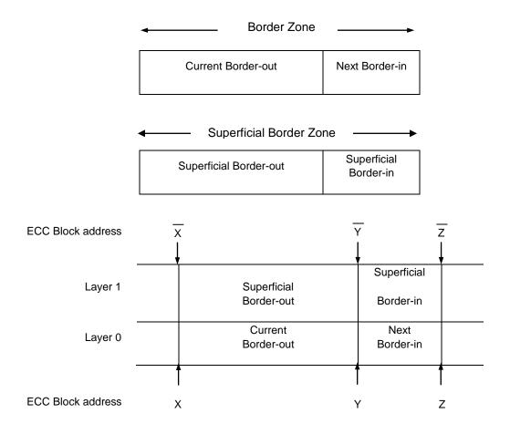
Figure L.1 — Structure of Border Zone
