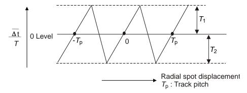
Figure 16 — Differential phase tracking error signal
