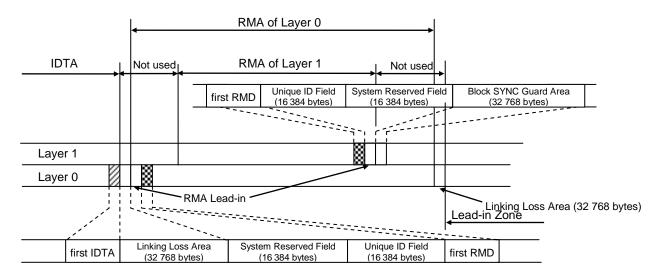
Figure 64 — Layout of the Recording Management Area
