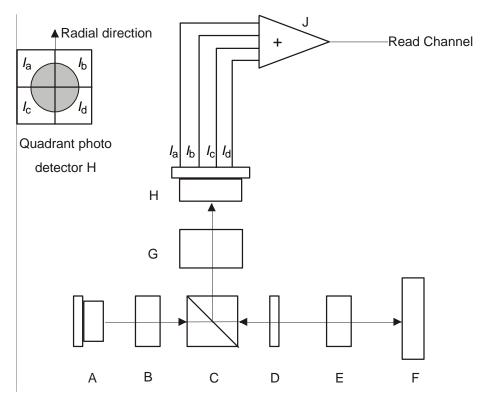
A Laser diode F Optical disk
