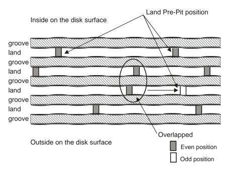
Figure 47 — Layout of land Pre-pit positioning
