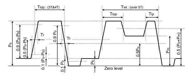
Figure 20 — Write pulse
