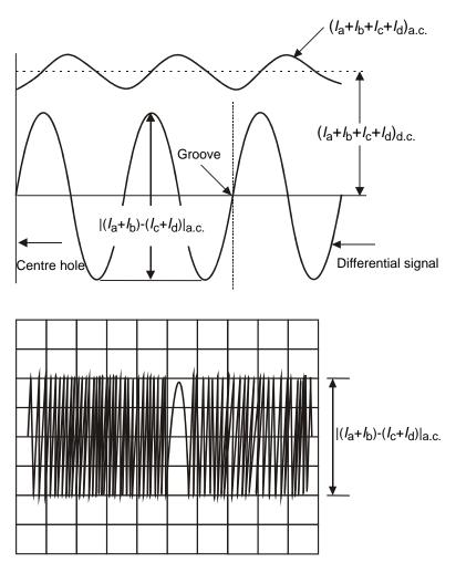
Figure 22 — Radial push-pull tracking error signal
