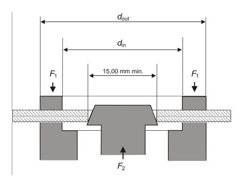
Figure A.2 — Clamping and chucking conditions
