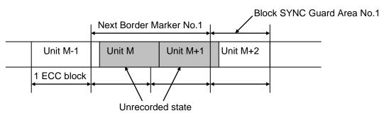
Figure L.4 — Structure of Next Border Marker
