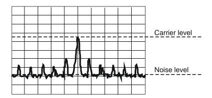
Figure 24 — Measurement of the wobble CNR
