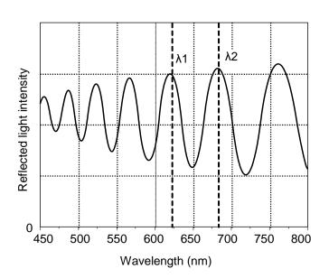
Figure R.1 — Space layer thickness measurement
