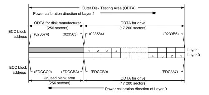
Figure 63 — Structure of Outer Disk Testing Area
