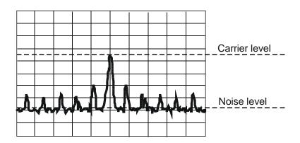
Figure 18 — Measurement of the wobble CNR
