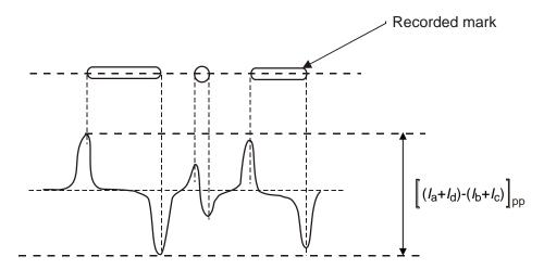
Figure 17 — Tangential push-pull signal
