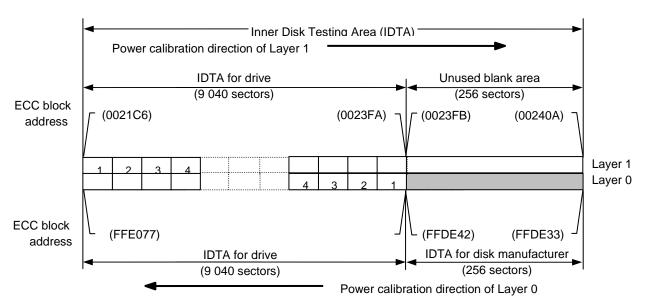
Figure 62 — Structure of Inner Disk Testing Area
