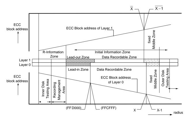
Figure 44 — Pre-pit sector layout and ECC Block numbering
