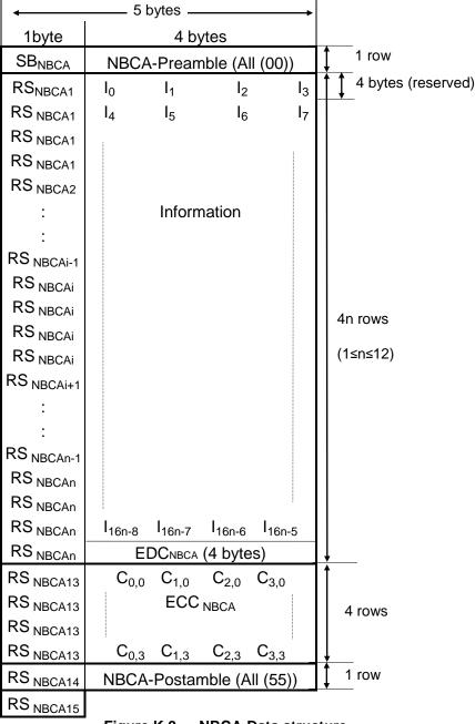
Figure K.2 — NBCA-Data structure
