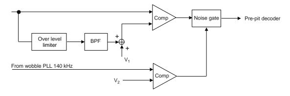
Figure M.2 — Example of the Land Pre-Pit detector
