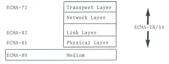
The Physical Layer provides the means for communication between Link Layer entities.
