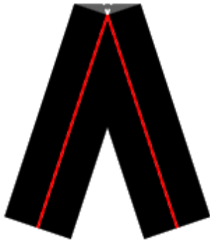
3 Figure 18–20. Beveled line join with obtuse angle
