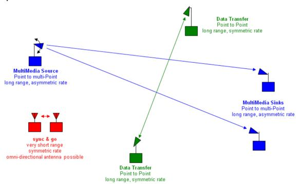
Since beacons, except the mode-D0 discovery beacons, are transmitted using directional antennas, they are broadcasted over a more confined area, thus resulting in a smaller "interference zone". Therefore, more links can be established simultaneously, thus enabling the spatial reuse of the channel time.
