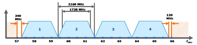
The standard specifies four frequency channels each with a symbol rate of 1.728 Giga-Symbols/second and with a separation of 2.160 GHz. All device types follow the same frequency plan. Under this frequency plan, the standard supports bonding of up to four adjacent channels. The channel bonding allows achieving higher data rates, or the same data rates while using smaller, more efficient constellations.
